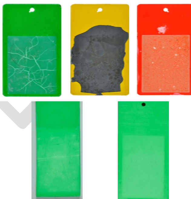
Figure 14 Test samples after artificial weathering (top paint / bottom plastic)
