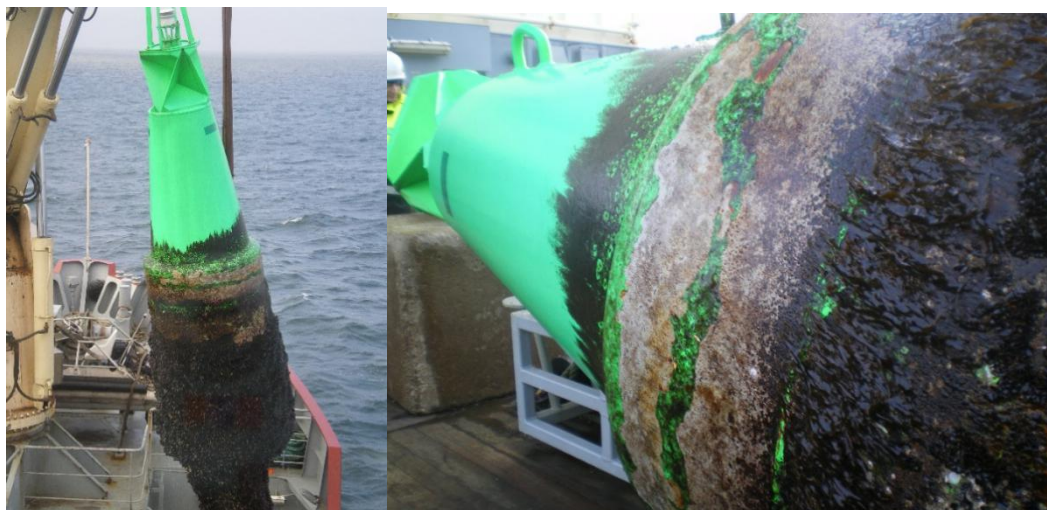
Figure 4 Coloured part with marine growth should be avoided when evaluating the fading of the colour but included when evaluating the visual day mark colour of the AtoN.
