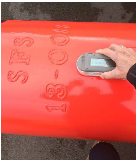
Figure 7 An example to use ID number of the buoy as a reference point (Datum)
